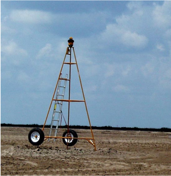
Tripod that carries the beam to the tractor used for laser leveling fields.
