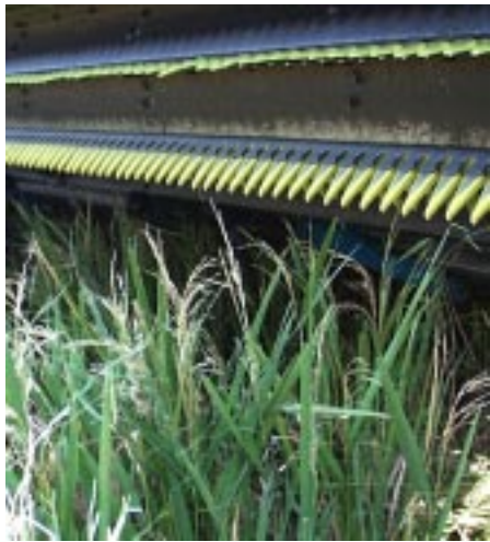
Close up shot of a stripper header showing the panicle remains after the grain has been harvested.
