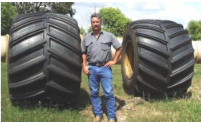
Balloon tires mean less compaction, especially important in a conservation tillage system.
