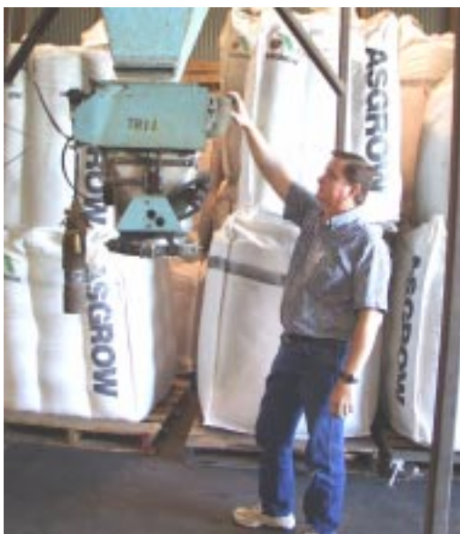
Foundation Seed Manager Robert Weatherton demonstrating the air-activated bagging scale used to package seed rice. The scale is inspected yearly by the TDA to insure accuracy.
