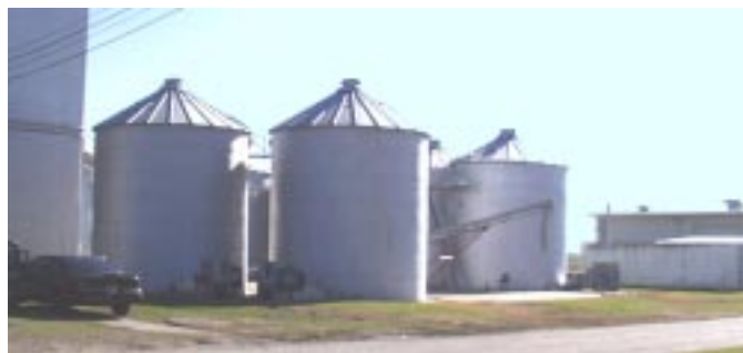
Storage bins for seed rice at the Texas A&M Research and Extension Center in Beaumont. The bins are carefully cleaned and treated after each use to prevent contamination of seed rice, and to prevent the spread of insect pests.
