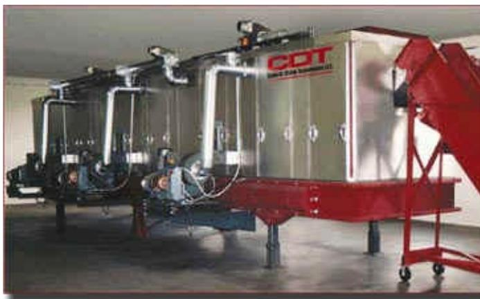
Catalytic Drying Technology's pilot scale test dryer – 4 ft. x 30 ft
