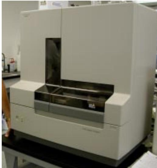
State of the art genetic analyzer, typically used for either DNA sequencing or genotyping. RiceTec uses it for genotyping microsatellite markers in rice. The system uses capillaries instead of a slab gel. They can run 16 samples in 40 minutes, and each sample may have from 1-8 markers multiplexed. Last year they produced 1.3 million data points using 3 machines, about 25,000 data points a week – or about 8,333 data points per machine per week.
