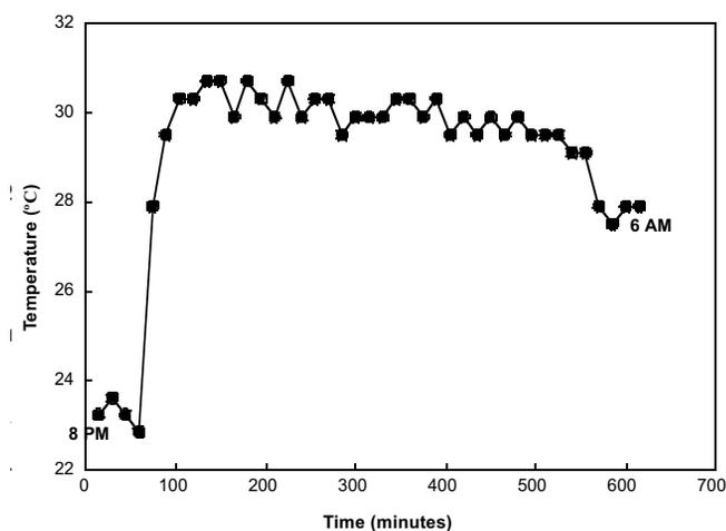
Daily trends of nighttime temperatures. The temperatures were maintained at 30°C (ambient plus 5°C) using infrared heaters. The nighttime temperatures were initiated 1h after the sunset until sunrise (8:00 pm to 6:00 am).
