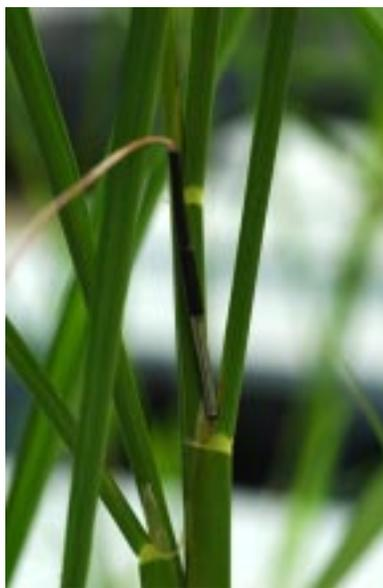
Pictured above is the hypodermic-like thermocouple that measures the internal temperature of the rice plant.
