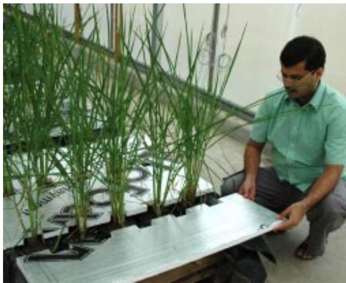
To minimize heating the water, which would confound the project's results, foam board insulation is cut to fit precisely around the rice plants.
