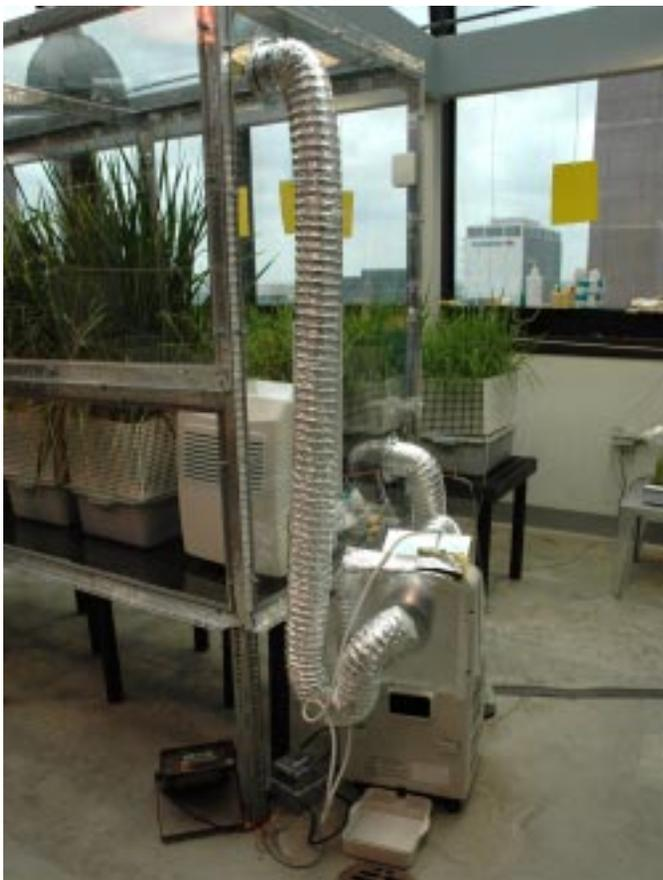
Growth chamber for growing Golden Rice with labeled hydrogen. The setup includes an air conditioning unit, fan, CO<sub>2</sub> supply and sensor, a dehumidifier and water-free air tank.
