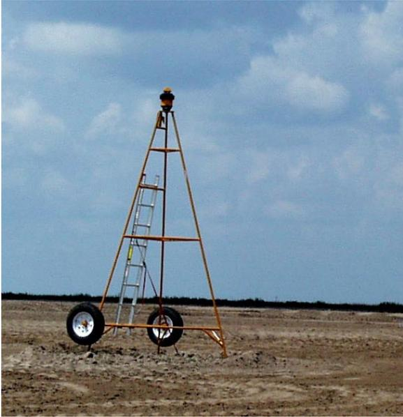
Tripod that carries the beam to the tractor used for laser leveling fields.
