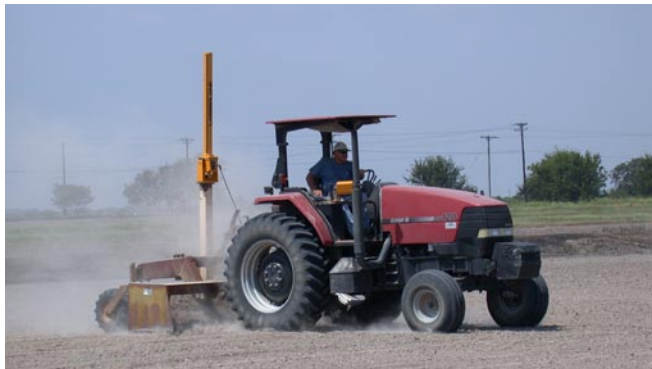
Eddie Pavliska, Farm Foreman, has worked at the Eagle Lake Station for over 20 years. Here he is shown laser leveling a research plot to improve water use efficiency.
